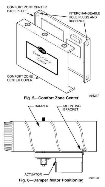
Before insulating the duct work, check for proper damper operation. Apply the 24vac between COM and OPN to open the damper and COM and CLS to close the damper. (See Fig. 7.) The damper will modulate counter-clockwise to open and clockwise to close.
